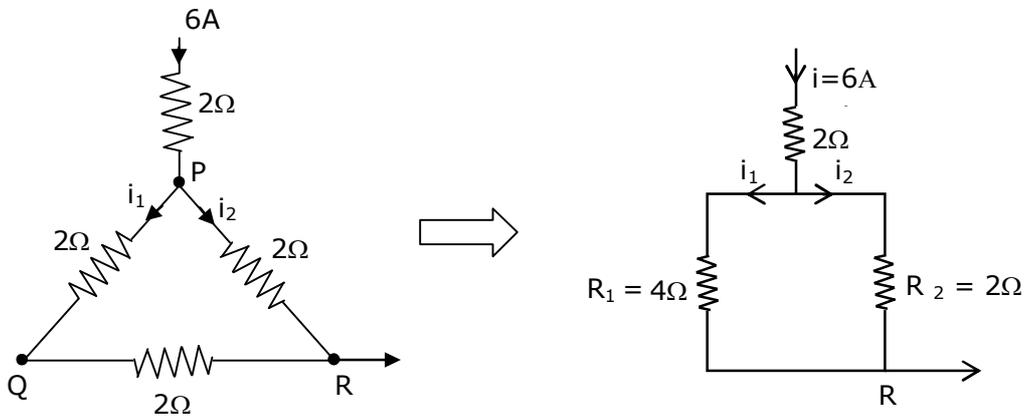
$$\text{The current } i_1 = \left( \frac{R_2}{R_1 + R_2} \right) i$$
