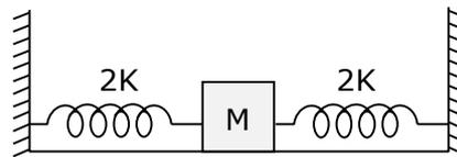
Due to parallel combination  $K_{\text{eff}} = 2k + 2k$
